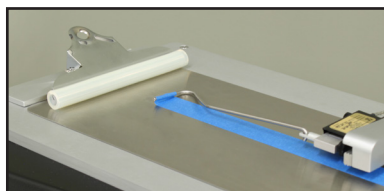
The 180 degree peel arm for peel testing is included with all FP-2265 units.
