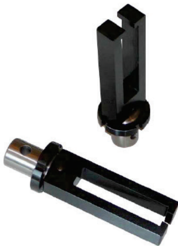
TA16-S18-Am32 according to ASTM D143 to test small clear specimens of timber
