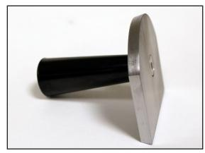
Template does not cut the pretest slit. This is cut by the ProTear prior to testing.
