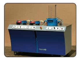
The SF-RK is an automatic sheet former used for the production of laboratory sheets in accordance to the Rapid Köthen method for measurement of the physical and/or optical properties of pulps.
