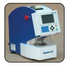
The BT-21 determines the bursting strength of paper, board and corrugated board. Two models are available to work with both light and heavy-weight materials. The BT-21 features steel frame body, strain gauge pressure transducer, pneumatic clamping system for the sample, built-in hydraulic system for the diaphragm, quick connector for calibration, built-in electronics and exclusive testing software.
