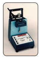
The 4171 tester measures the force required to bend a variety of materials under controlled and repeatable conditions. This force may be equated to stiffness, resilience, flexibility or pliability depending on the nature of the materials and purpose of the test. This digital bending resistance/stiffness tester can be equipped with a parallel clamp and tubing clamp and connects to a computer via RS-232.
