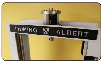
▲ QC-3A Load Cell Adapter (Part No. 771-3000) can be ordered to move the load cell outside of the frame to add extra crosshead travel.
