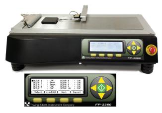
This coefficient of friction (COF)/peel tester can measure static and kinetic coefficient of friction, as well as run seal strength tests, 180° peel, 90° peel and T-peel tests. The
