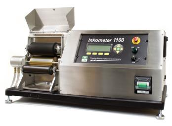
The Inkometer 1100 consists of three rollers. The center roller is a temperature controlled brass roller. The bottom roller is an oscillating rubber composition distribution roller. The top roller is a rubber composition roller attached to the measuring system which measures tack. Rollers are available for testing standard and UV inks. The brass roller temperature is controlled by circulating a coolant mixture provided by a Constant Temperature Circulator (CTC).
