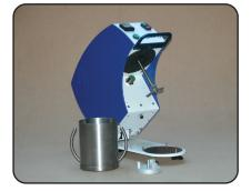
The DSG is vital for laboratory wet disintegration of pulp and the correct preparation of pulp and pulp suspensions. It eases the disintegration time by up to 87% compared to standard models.
