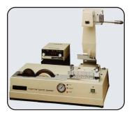
**Applications צ** Paper, Paperboard The 1314 Internal Bond Tester utilizes the Scott Method to produce a high speed Z-Directional rupture of paper and paperboard. It is a dynamic test that measures and defines strength in terms of energy absorption. The Internal Bond Tester is ideal for monitoring the effects of dry strength additives and to evaluate stock preparation and refining.
