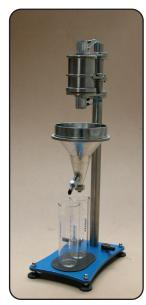
The CF-21 Canadian Freeness is used to determine the drainability of pulp suspensions. The drainability is the measurable index of the efficiency of refining process.
