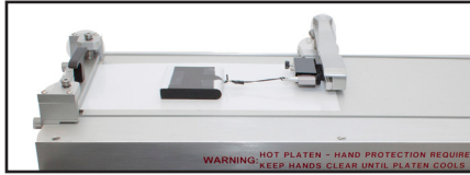
Heated Platen - Temp Range 21°C to 176.7°C (70°F to 350°F)
