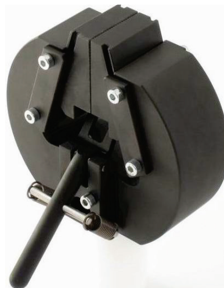
TAS622-BP: Pyramids 1x45°, hardened steel
