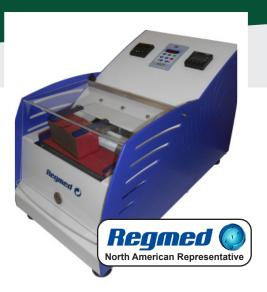
▲ The Ink Rub Tester determines the abrasion resistance of printed materials.
