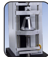
Ball Burst ASTM D6797
