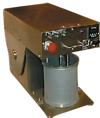
▲ T-100 Pulp Disintegrator prepares samples to TAPPI and ISO standards
