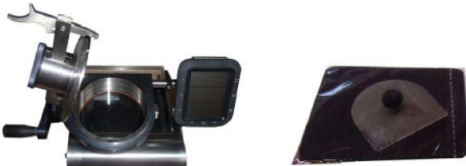
In order to complete the Cobb test you will also need blotting papers from 200 to 250g/m<sup>2</sup> and an analytic scale with an accuracy of 0.001g.
