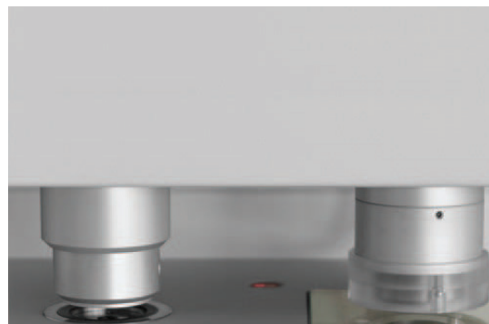
▲ Testing heads for air permeability and roughness with photo detection cell
