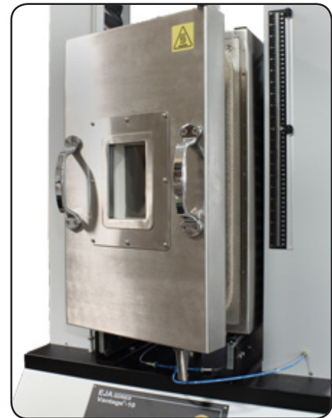
▲ The environmental chamber mounted on dual column Vantage-10 tester to measure the affects of elevated temperatures on material performance.
