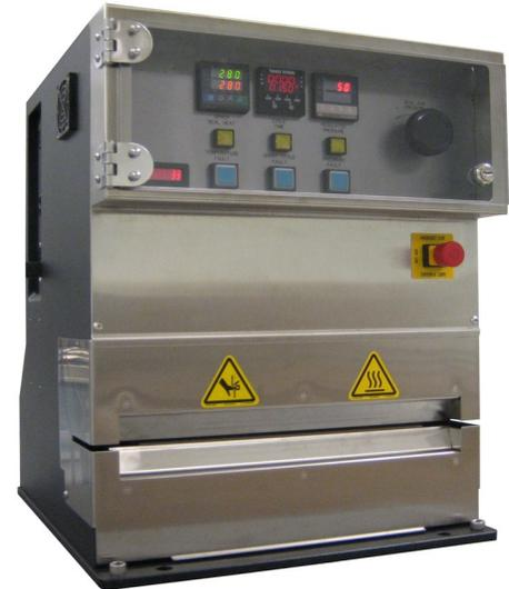
**Short Cycle Indicator** disables the sealer if a seal cycle is terminated before the entire dwell time has fully elapsed, indicating to the operator that the last seal cycle was incomplete.
