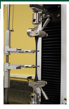
▲ The Extensometer enables the measurement of highly elastic materials with Thwing-Albert's Vantage.
