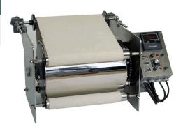
▲ The Drum Dryer is ideal for drying hand sheets over a wide range of dimensions.
