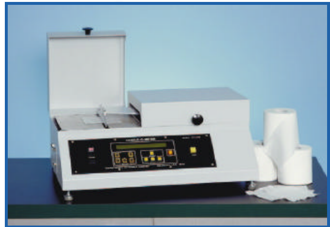
▲ Handle-O-Meter measures the combined effects of flexibility and surface friction of sheeted materials.
